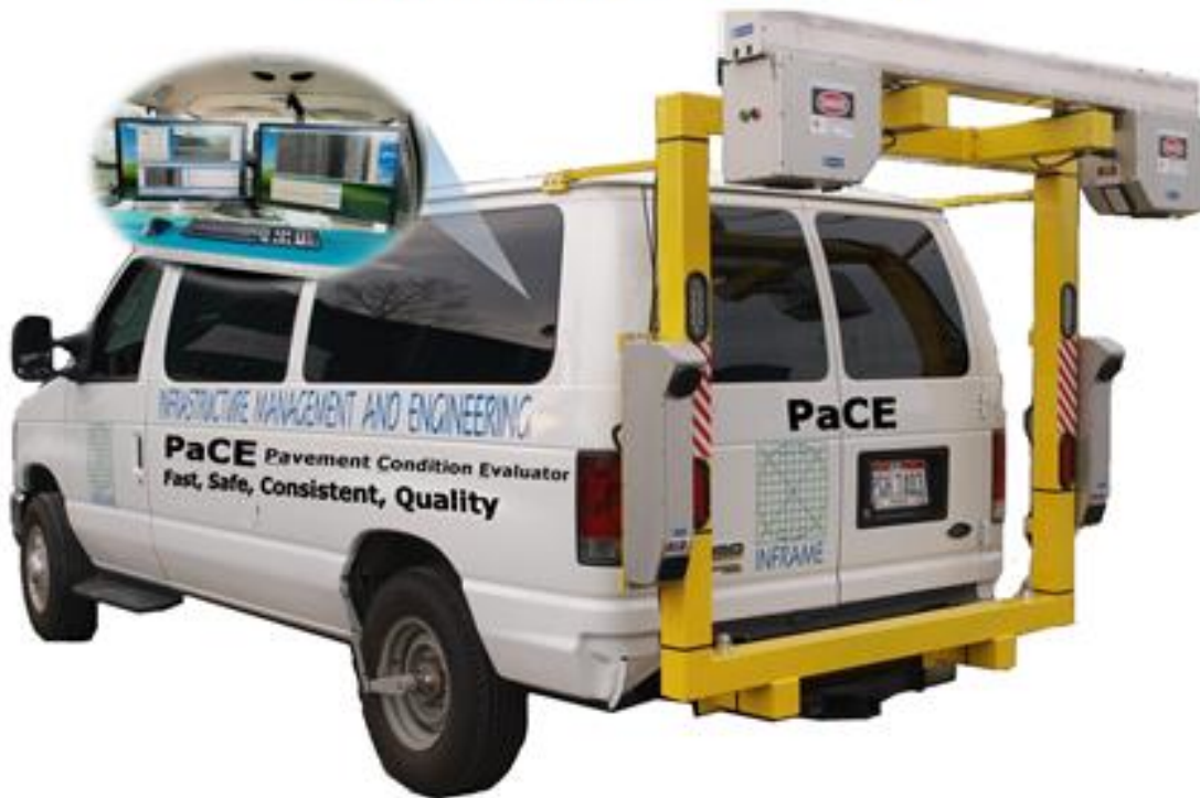
Figure 1 Pavement Condition Evaluator, PaCE
