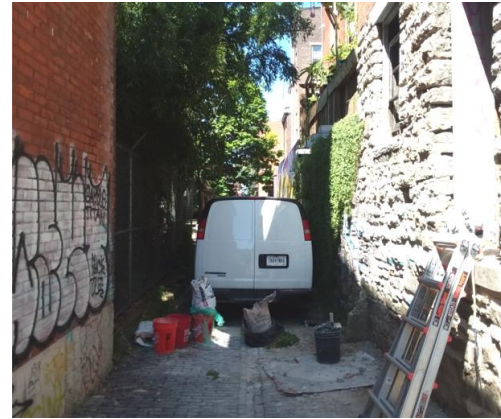
8.5' wide and obstructed Bolivar Alley is too narrow for navigation and for fire trucks to fight fires at the rear of 12th and 13th Street buildings.
