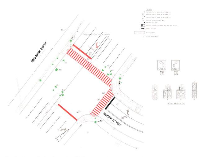
Developer's roadwork will consist of infrastructure improvements at the intersection of Red Bank Expressway and Medpace Way on the west side of the Medpace Campus. The eligible roadway improvements include new pavement markings, adjustment of the existing elevated medians to allow for proper vehicle movement, and a new traffic signal. Accordingly, Developer shall cause the completion of all of the following with respect to the Intersection Improvements at the Intersection Improvement Site:
