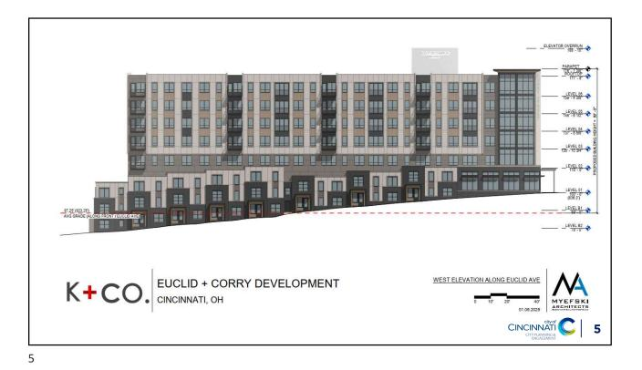
ELEVATOR OVERRUN **Euclid & Corry** 89' - 95' in height • ROOFTOP 170 - 185 units (460-500 beds) ٠ -205 - 225 vehicle parking spaces LEVEL 06 I 180 - 215 bicycle parking spaces LEVEL 05 LEVEL 04 LEVEL 03 LEVEL 02 T EVEL 01 100' - 0" 💠 (836.0') LEVEL B1 87.25 (823.25) AVG GRADE (A AVE) \_LEVEL 82 WEST ELEVATION ALONG EUCLID AVE EUCLID + CORRY DEVELOPMENT K+CO • CINCINNATI, OH ARCHITECTE 01.08.2025 6
