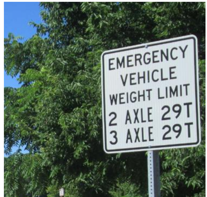
Current Load posting signs for bridges in Ohio.
