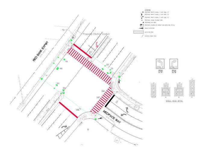
Developer's roadwork will consist of infrastructure improvements at the intersection of Red Bank Expressway and Medpace Way on the west side of the Medpace Campus. The eligible roadway improvements include new pavement markings, adjustment of the existing elevated medians to allow for proper vehicle movement, and a new traffic signal. Accordingly, Developer shall cause the completion of all of the following with respect to the Intersection Improvements at the Intersection Improvement Site:
