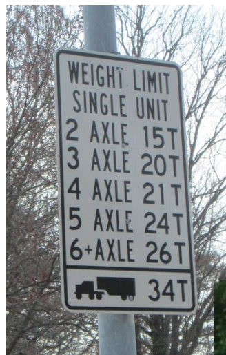
Current Load posting signs for bridges in Ohio.
