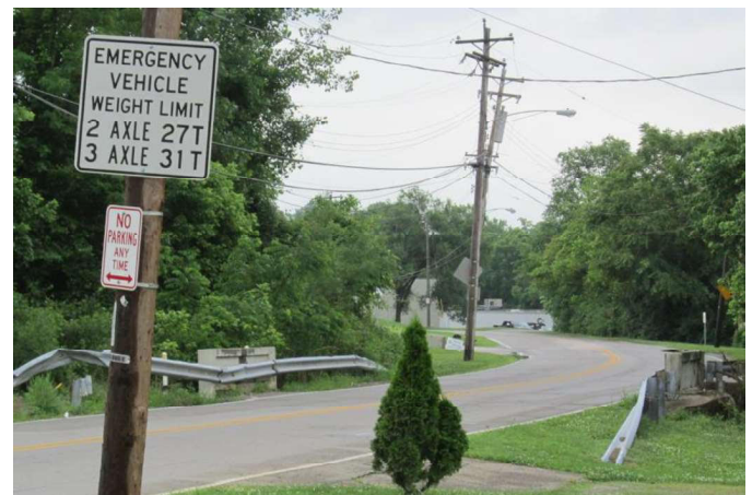
Current Load posting signs for bridges in Ohio.
