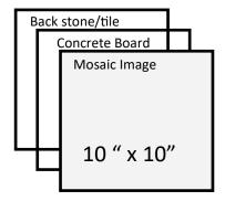
Others mosaic game squares (see image above) will be **mounted indirectly to** fencing and existing sign posts. These tile images will be attached to concrete board when they are proposed as signs. The width of the squares will vary as the tile width varies, but will be 1.5-2 inches thick. The back of the concrete board would be painted and sealed, or have a large stone or porcelain tile mortared to the back. These flat mosaics would be bolted or screwed to:
